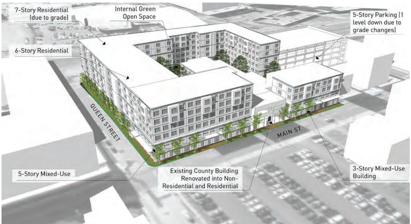
Figure 74: Conceptual View of Preferred Development Plan for DHA Office and Criminal Justice Building Site
