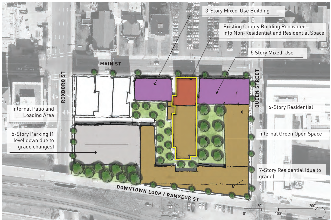
Figure 73: Proposed Preferred Development Plan for DHA Office and Criminal Justice Building Site
